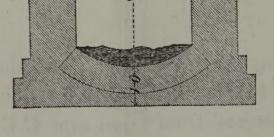
3. There are six man-holes to the main sewer through the New Palace, marked M on the plan, there being one situated in each court-yard. The accompanying section exhibits the form of the sewer. It is five feet six inches in height by three feet in width. 3. These man-holes are, and always will be, kept closed and air-tight, except when occasionally opened for repairs on the examination of the main sewer.
